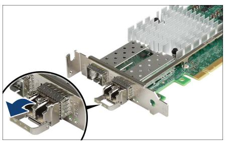
Figure 43: Unlatching the locking bail
